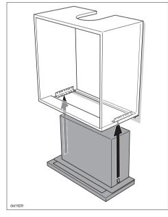
Lift the appliance up into the housing from below, and engage in the brackets.
